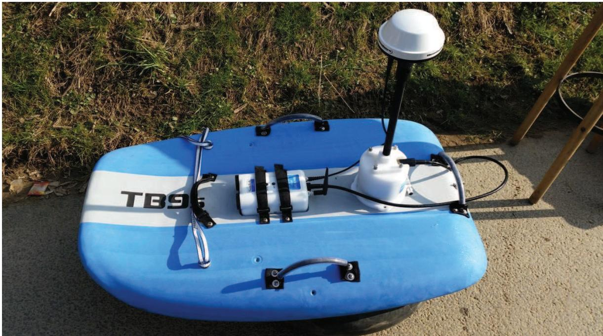
Appareil de jaugeage SONTEK Riversurveyor M9
