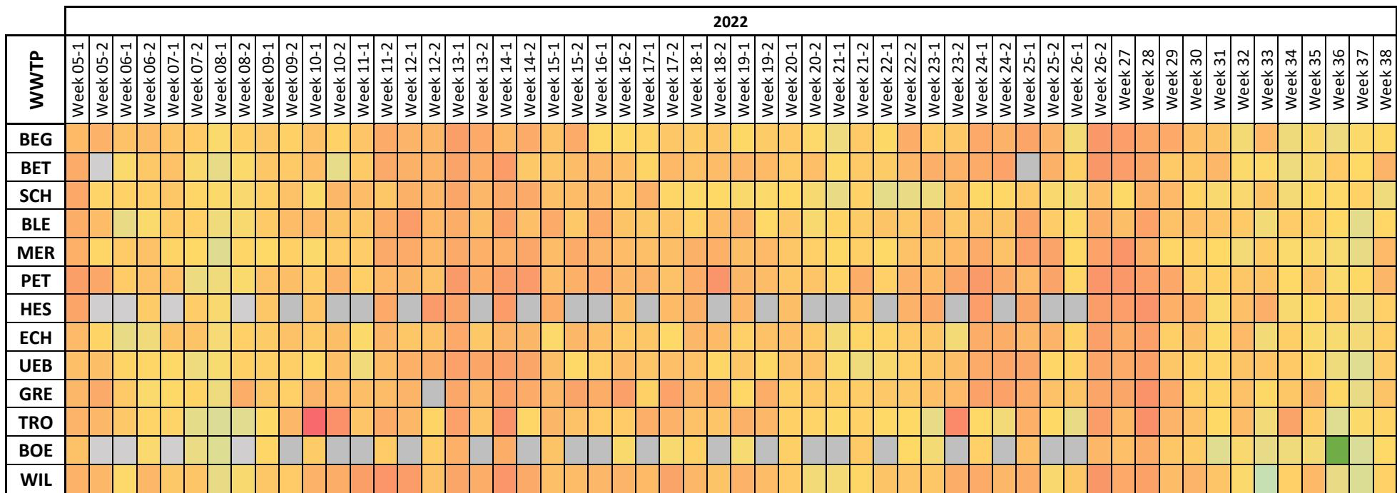
Figure 2a – RT-qPCR quantification time-course monitoring of SARS-CoV-2 (*E* gene) in the four most impacted wastewater treatment plants from March 2020 to September 2022. Grey squares: daily confirmed cases for the contributory area of each wastewater treatment plant, dots: SARS-CoV-2 flux (RNA copies / day / 10 000 equivalent inhabitants).
