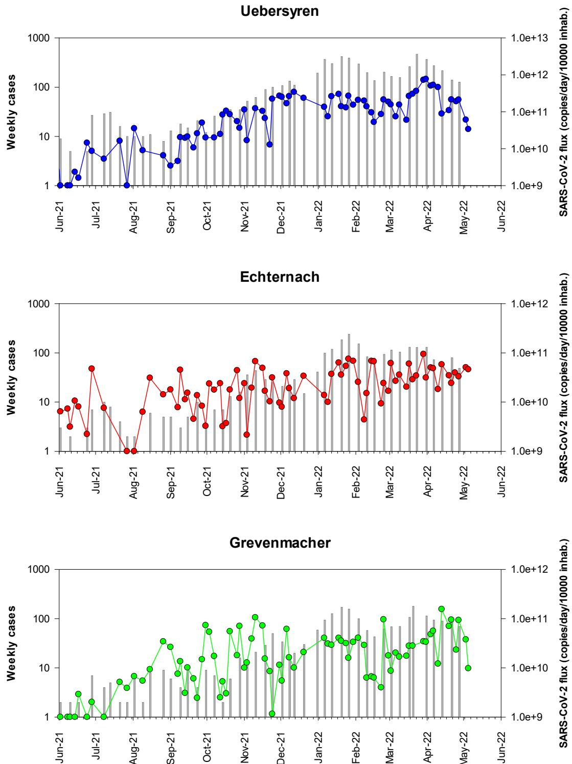
Figure 5a – RT-qPCR quantification time-course monitoring of SARS-CoV-2 (E gene) in SIDEN wastewater treatment plants from May 2020 to May 2022. Grey squares: daily-confirmed cases for the contributory area of each wastewater treatment plant, dots: SARS-CoV-2 flux (RNA copies / day / 10 000 equivalent inhabitants)
