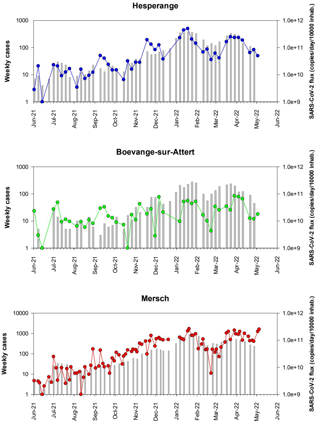
Figure 4a – RT-qPCR quantification time-course monitoring of SARS-CoV-2 (E gene) in SIDEST wastewater treatment plants from May 2020 to May 2022. Grey squares: daily-confirmed cases for the contributory area of each wastewater treatment plant, dots: SARS-CoV-2 flux (RNA copies / day / 10 000 equivalent inhabitants).
