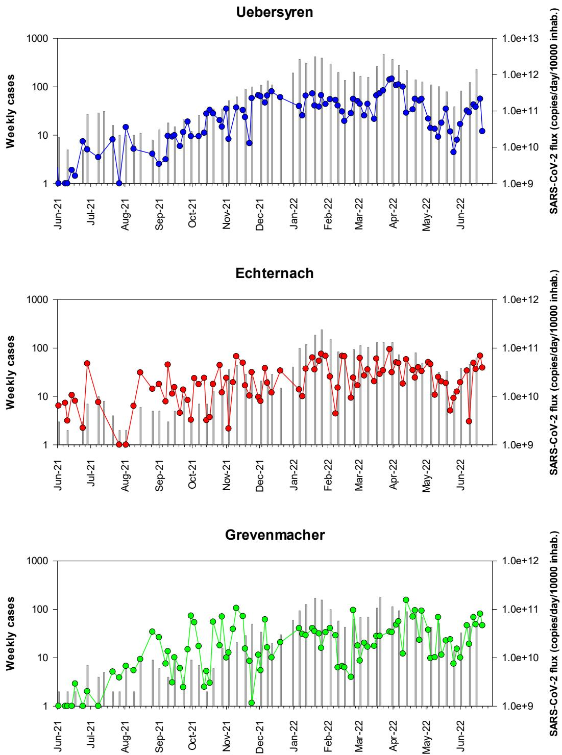
Figure 5a – RT-qPCR quantification time-course monitoring of SARS-CoV-2 (E gene) in SIDEN wastewater treatment plants from May 2020 to June 2022. Grey squares: daily-confirmed cases for the contributory area of each wastewater treatment plant, dots: SARS-CoV-2 flux (RNA copies / day / 10 000 equivalent inhabitants)
