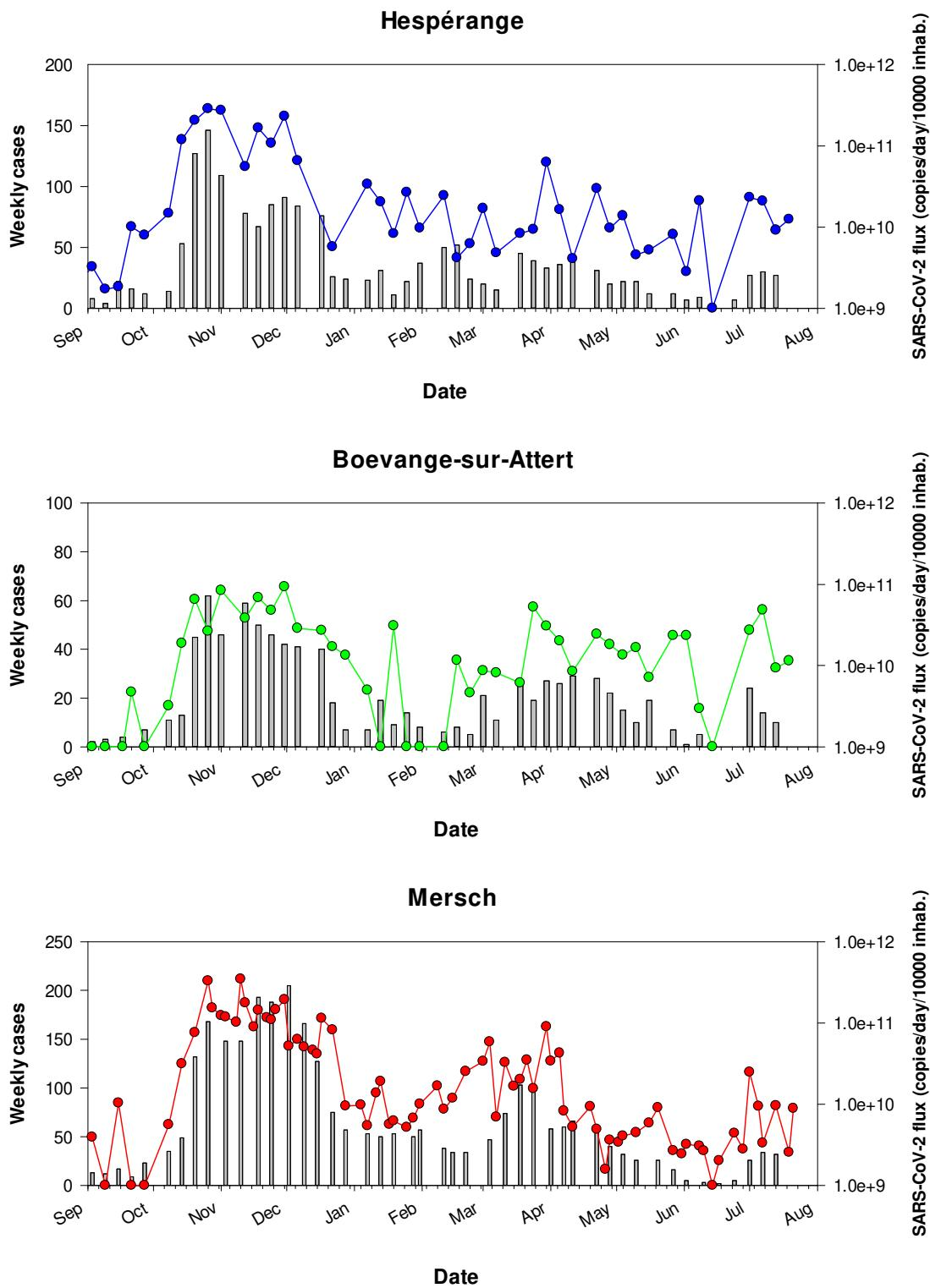
Figure 4a – RT-qPCR quantification time-course monitoring of SARS-CoV-2 (E gene) in SIDEST wastewater treatment plants from March 2020 to July 2021. Grey squares: daily-confirmed cases for the contributory area of each wastewater treatment plant, dots: SARS-CoV-2 flux (RNA copies / day / 10 000 equivalent inhabitants).
