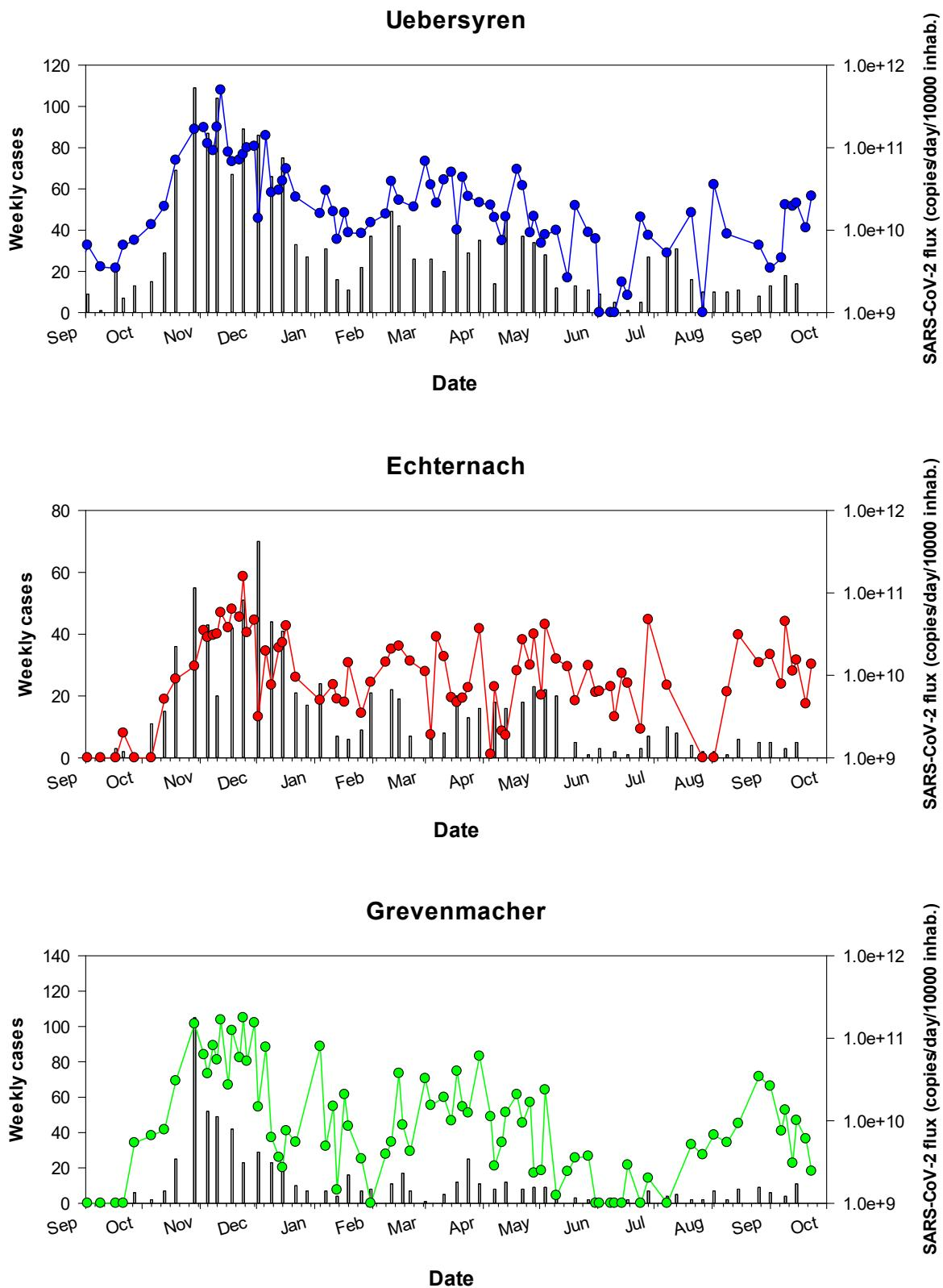
Figure 5a – RT-qPCR quantification time-course monitoring of SARS-CoV-2 (E gene) in SIDEN wastewater treatment plants from March 2020 to Septembe 2021. Grey squares: daily-confirmed cases for the contributory area of each wastewater treatment plant, dots: SARS-CoV-2 flux (RNA copies / day / 10 000 equivalent inhabitants)
